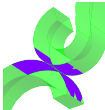
Plot of solver-based no penetration contact. Rendering of mesh elements that participate in contact formulation.
